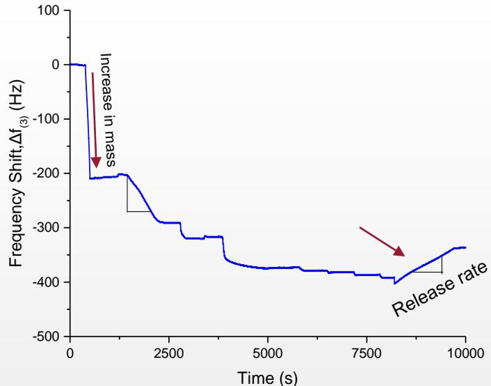
Figure: Calculation of initial deposition rate from frequency shift slope
