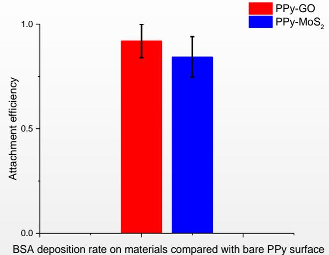
Figure: Maximum deposition (left) and attachment efficiency (right) of BSA on PPy, PPy-GO and PPy-MoS<sub>2</sub> surfaces without any potential.
