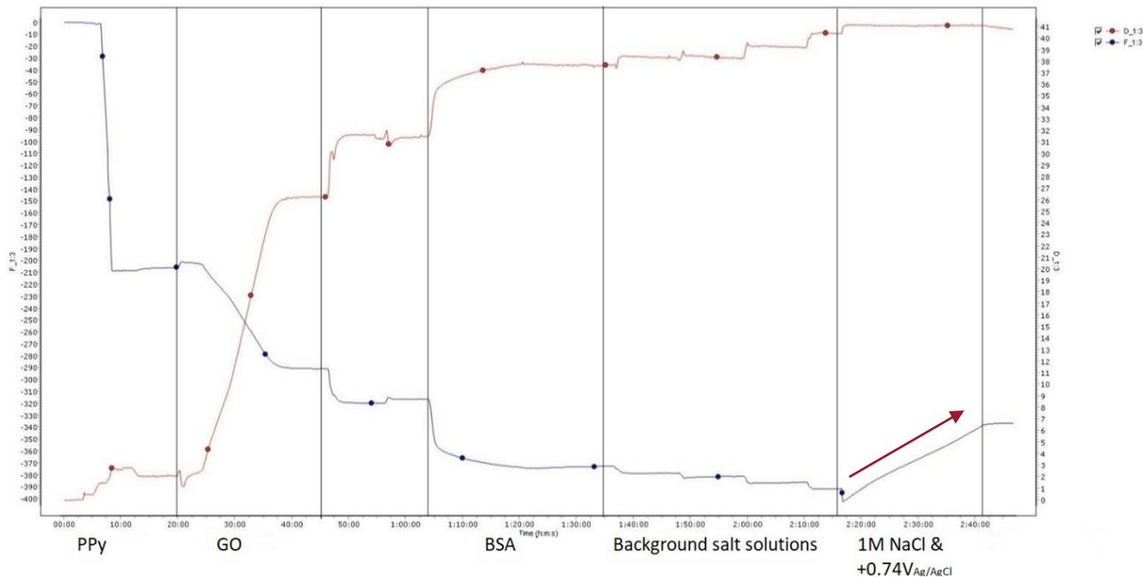
Figure: Removal of BSA from PPy-GO surface by 1M NaCl electrolysis under +0.74V<sub>Ag/AgCl</sub>.
