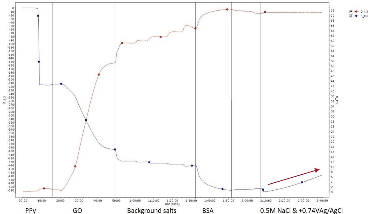
Figure: Removal of BSA from PPy-GO surface by 0.5M NaCl electrolysis under +0.74V<sub>Ag/AgCl</sub>.
