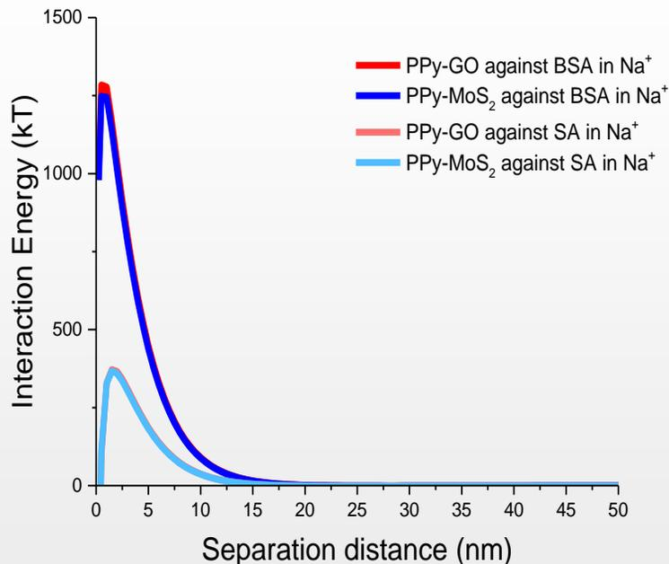
Fig: High energy barrier prevents the BSA/SA coming into true contact of GO and MoS<sub>2</sub>
