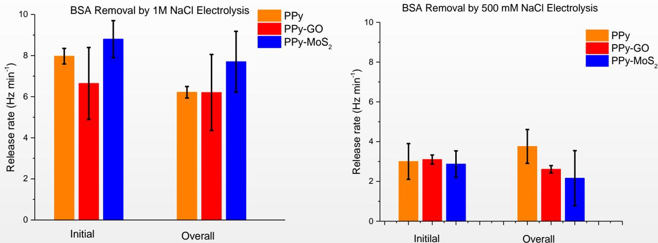
Figure: Release of BSA from PPy, PPy-GO and PPy-MoS<sub>2</sub> surfaces in presence of 1M NaCl (left) and 0.5M NaCl (right) under +0.74V<sub>Ag/AgCl</sub>
