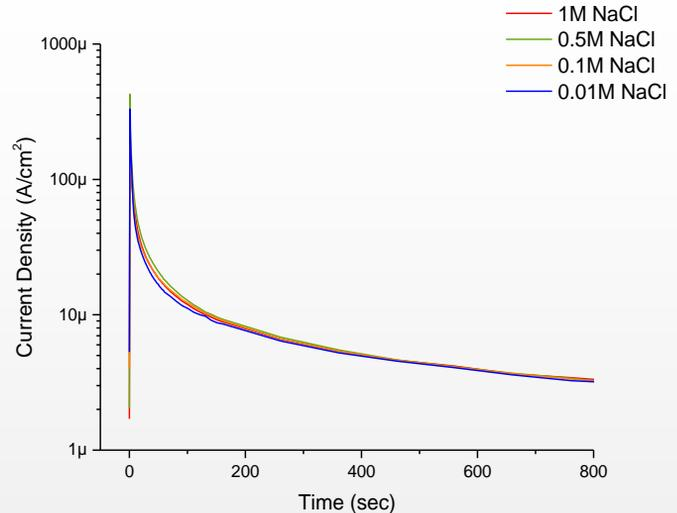
Figure: Generation of anodic current on material surfaces indicates the electrochemical reaction going on the working electrode when  $+0.74\text{V}_{\text{Ag}/\text{AgCl}}$  was applied.
